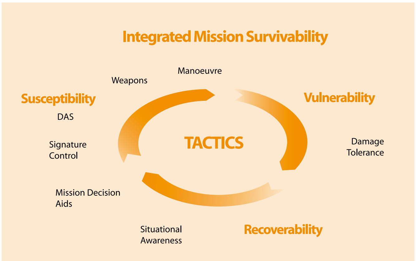
Figure 3. Survivability may be broken down into three elements: susceptibility vulnerability and recoverability
