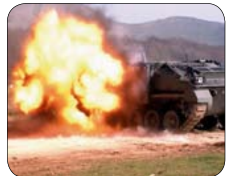
Electric armour defeating an RPG
