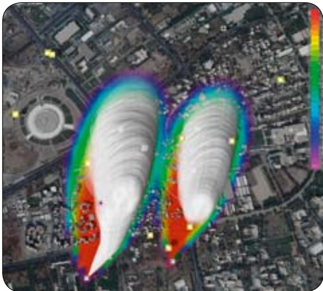
Output from Urban Dispersion Model showing spread of CW agent
