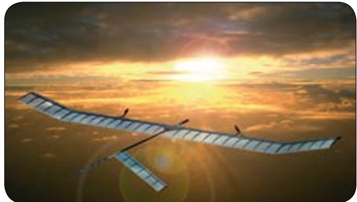
Zephyr, solar powered unmanned air vehicle
