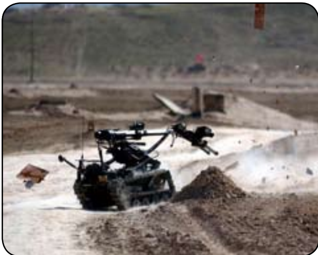
Explosive ordnance disposal using a remotely operated vehicle in Afghanistan
