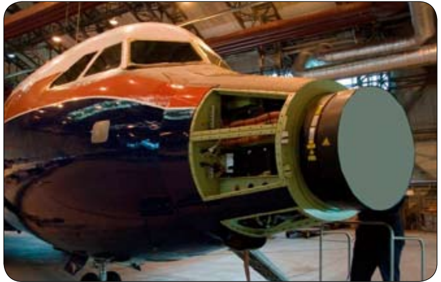
Captor Active Electronically Scanned Array Radar on BAC1-11 (Selex)
