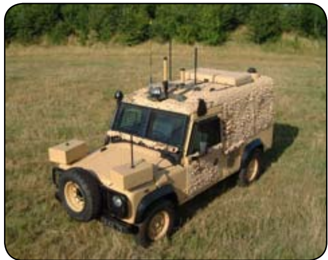
Snatch Landrover fitted with an electronic countermeasures suite as part of an Urgent Operational Requirement
