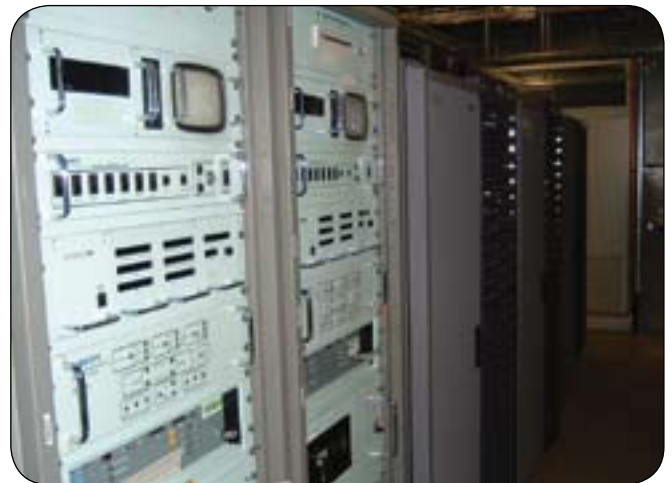
The 'Generic Acoustic Processing System' used for analysis of sonar data
