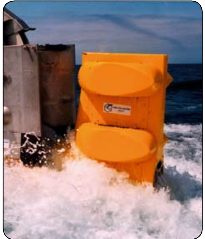
Sonar 2087, an advanced sonar upgrade fitted to HMS Westminster
