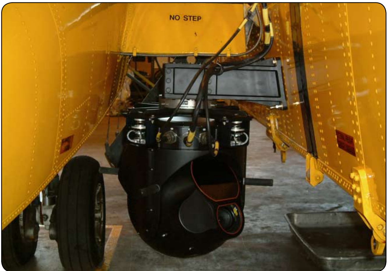
Electro-optic infra-red turret fitted for airbourne surveillance
