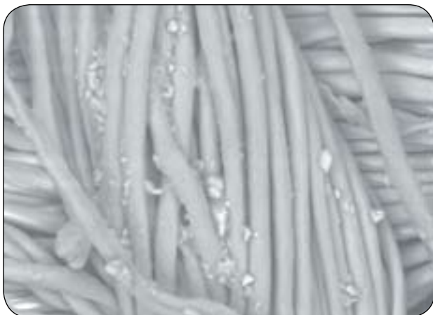
Semtex print on fine cotton fabric at x500 magnification
